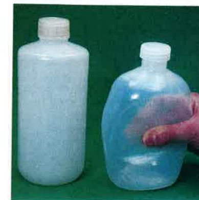
Two polyethylene bottles. The one on the left is made with high-density polyethylene, while the one on the right is made with low-density polyethylene.
